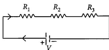
The two or more resistances are said to be connected in series if the current flowing through each resistor is the same.
